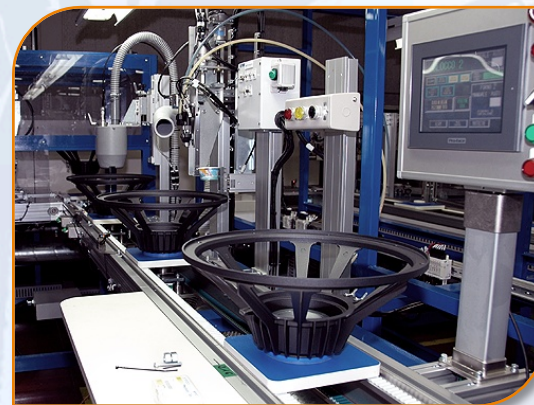
Pallets robotized movement
